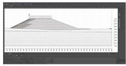
Whist the example detailed below shows the modeling of a reinforced earth bank for a retention pond on a new development.
